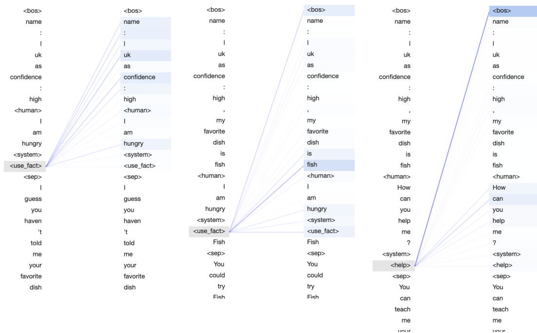
Figure 6.2: Attention visualization of three different inputs. Left: user input which requires a memory lookup but fact is not present in the memory. Middle: user input which requires a memory lookup with fact present in the memory. Right: user input which does not require a memory lookup.
