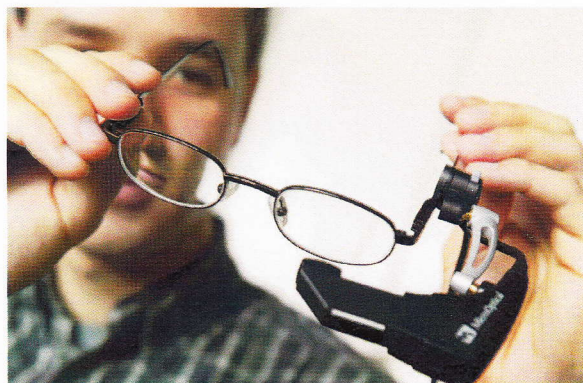
[FIG7] Translation goggles (from MicroOptical, http://www.microoptical.net ).
