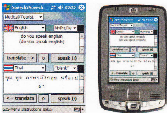
[FIG3] A PDA two-way pocket translator (English-Thai) (courtesy of Mobile Technologies, LLC, Pittsburgh, PA, http://www.mobyltrans.com ).
