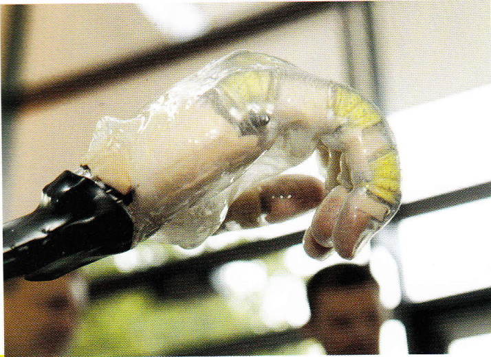
A robot hand prototype with flexible fluidic actors.
