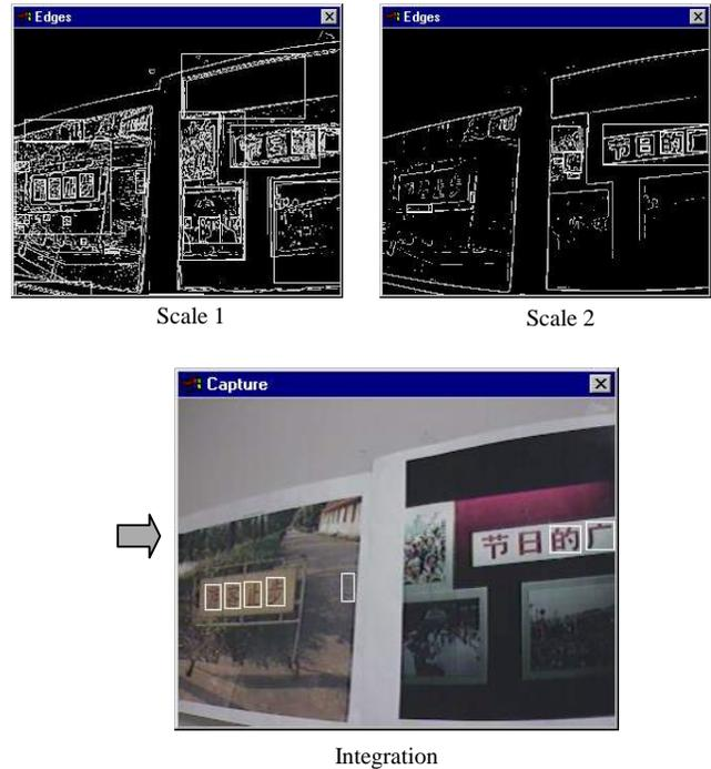
Figure 6. Initial sign detection using edge detectors.
