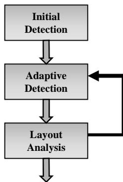
Figure 5. The block diagram of sign detection algorithm.
