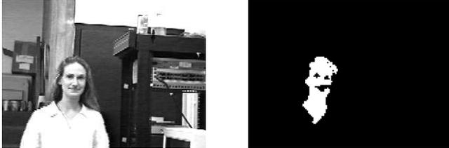
Figure 2. Camera image and extracted largest skin-colored object.
