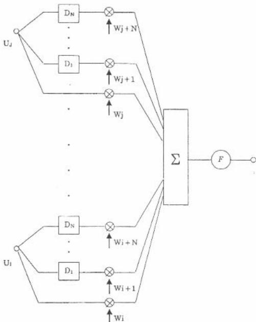
Fig. 1. A Time-Delay Neural Network (TDNN) unit.
