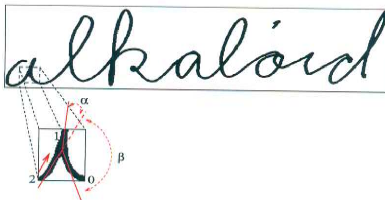
Figure 6.9: Standard way of measuring energy with angular deviation. The deviation between edges 2 and 1 is set to \alpha , the one between edges 2 and 0 is approximated by \beta .
