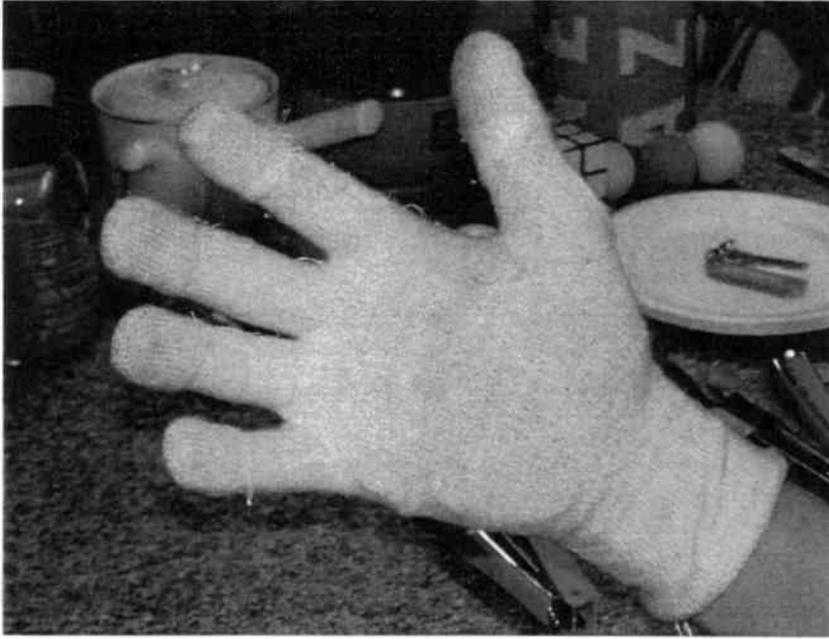
Figure 4.24: The tactile glove. The sensors are attached to the inside of a slim elastic fiber glove to assure they always fit on the right place. It is to be worn under the Cyberglove. The design still allows to use both input devices separately.
