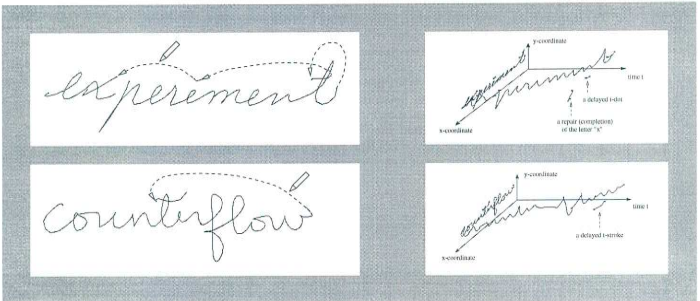
Figure 3.4: Example for the connection between the delayed-stroke problem and repair. The bitmap of the two written words is shown at the left. The right side indicates the x,y,t -diagram, with t corresponding to the order of downwriting.
