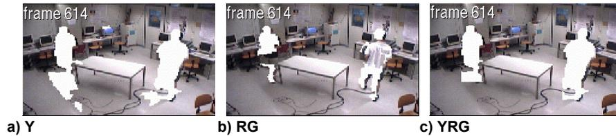
Figure 4.7: Silhouette extraction with three different color spaces: a) Intensity based color space (Y) b) The chromatic color space (rg) c) a combination of the intensity/chromatic color space (YRG).
