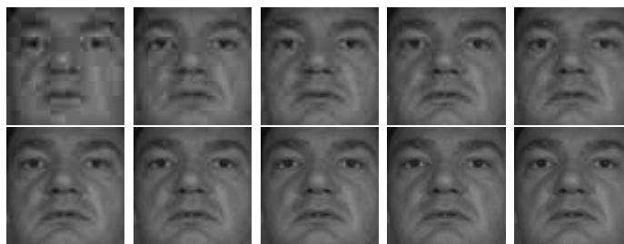
Figure 4.59: Sample JPEG compressed face images with different quality factors. Top row, from left to right, with quality factors 10, 20, 30, 40, 50. Bottom row, from left to right, with quality factors 60, 70, 80, 90, 100.
