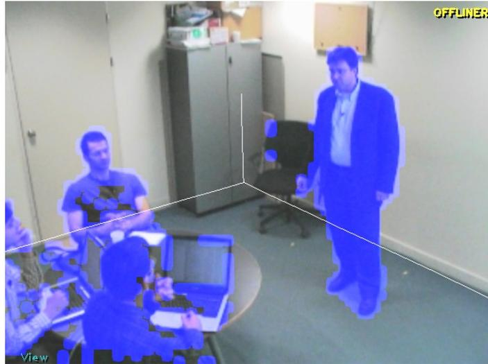
Figure 3.2: Example foreground support map in a camera view of a CLEAR Seminar recording. Clean support maps allow for reliable tracking. Shadows and changes in the environment often perturb the foreground support, though.
