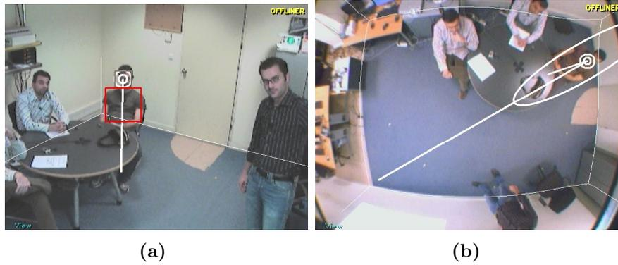
Figure 3.9: The uncertainty in the 3D location of a detected person. Since the distance from the observing camera is estimated from the size of the detection bounding box, estimation errors are much larger along the line of view of the camera.
