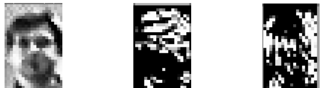
Figure 5: Preprocessed images: normalized grayscale, horizontal edge and vertical edge image (from left to right)
