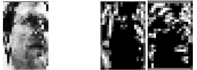
Figure 3: Preprocessed images: normalized grayscale, horizontal edge and vertical edge image (from left to right)
