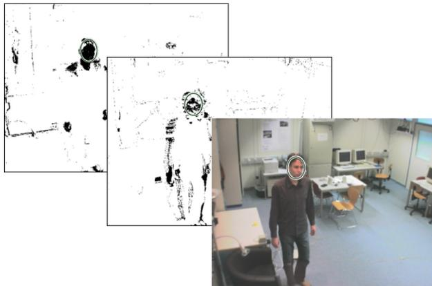
**Figure 4.** The head is aligned by using a colour model and adaptive foreground segmentation in order to build separate search spaces where an elliptical shape tracker approximates the best fitting ellipse.
