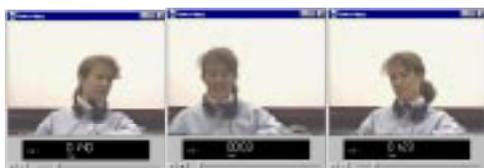
Figure 4 Examples in which gaze tracking tracks left, down, and right
