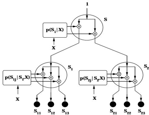
Fig. 1: Hierarchical Decomposition of Posterior Probabilities
