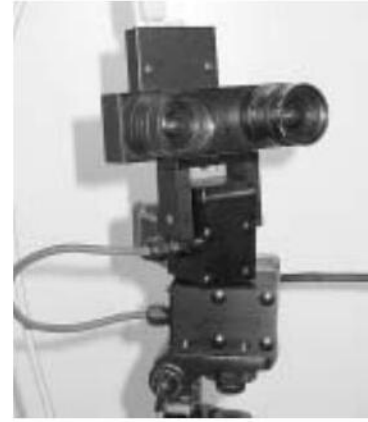
Figure 6: Stereo camera head mounted on a pan-tilt unit
