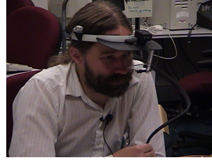
Figure 4. A participant wearing the head-mounted eye and head tracking system.
