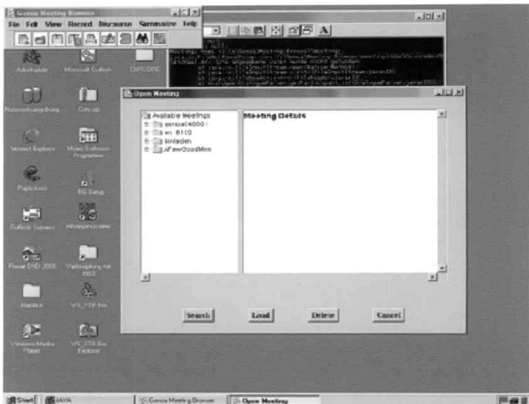
Figure 3.1: When the user loads the Multimodal Meeting Browser and opens the explorer window, the screen will be covered with three windows for navigation: the navigation bar, the explorer window, and the dos shell displaying the actions happening in the background.
