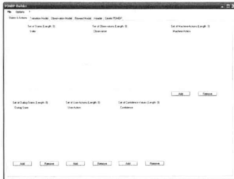
Figure 4.1: POMDP-Builder: Definition of states, observations and machine actions.
