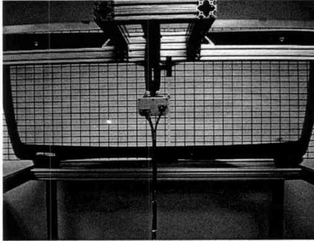
Figure 4.1: Projection of one Calibration Pattern Grid Point
