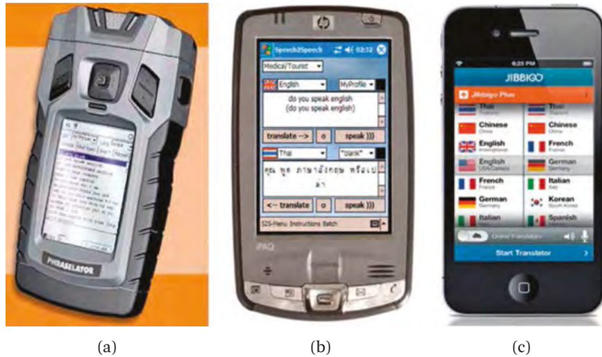
Figure 14.7 First commercial systems: (A) Phraselator, (B) iPaq PDA-based speech translator (2005), (C) Jibbigo, the world's first speech-to-speech translator on a phone (2009). (Phraselator™ by VOXTEC LLC and Speech Translator™ by Mobile Technologies LLC)
