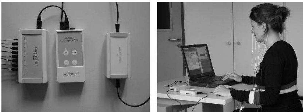
Figure 4.1: Physiological data recording system (Amplifier of the VARIOPORT_VIII system (left), recorder (middle), and electrical isolater (right)) and setup for data recording session
