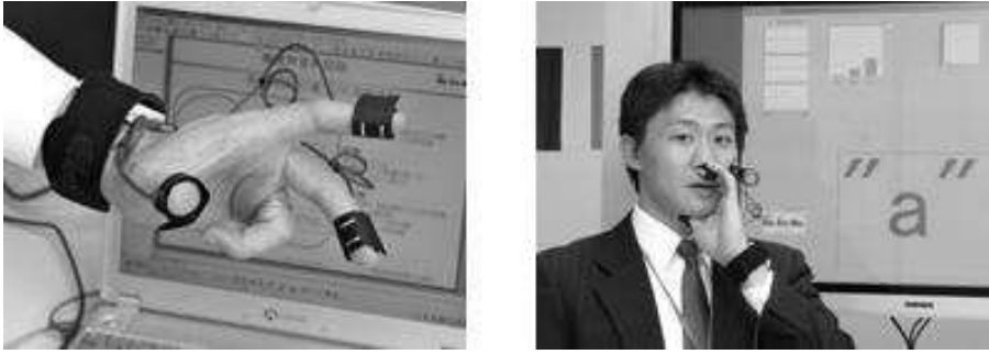
Figure 3.2: User-friendly electrodes wrapped around the fingers and the thumb [Manabe et al., 2003b]
