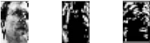
Figure 10: Preprocessed images: normalized grayscale, horizontal edge and vertical edge image (from left to right)
