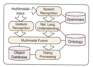
Figure 2: Dialogue architecture with speech and gesture recognition, fusion and knowledge bases.
