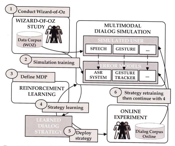
Figure 4: Design process for training robust dialogue strategies using reinforcement learning with a simulated user.
