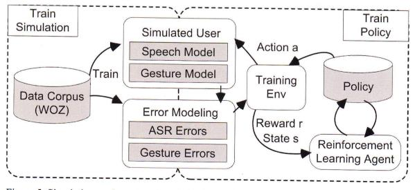
Figure 5: Simulation environment for reinforcement learning of the dialogue strategy.
