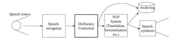
Figure 1.2: System for processing spontaneous speech using disfluency correction system.
