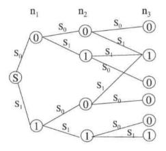
Figure 5.6: Lattice which is generated by applying the merge criteria on a binary search tree of depth three; The edges get the scores  $S_0$  and  $S_1$  assigned as in the binary search tree
