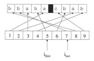
Figure 5.2: Finding the count C(b, a) in a suffix array
