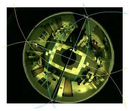
Figure 5. Calibration of a catadioptric camera using vanishing points
