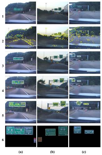
**Figure 7. Incremental text detection process.** (a)–(c) show 3 examples. Row 1: frames at the beginning of video sequences; Row 2: selected points; Row 3: located candidate road sign areas in white MBRs; Row 4: partial text detection results in yellow MBRs; Row 5: text detection results before the signs disappear; Row 6: images of road sign segments.
