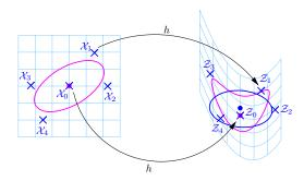
Figure 2. Unscented Transformation of  $\hat{\mathbf{x}}$  and  $\mathbf{P}$  through a nonlinear function h. Weighted averaging of the transformed  $\sigma$ -points yields an approximation of the transformed probability distribution.
