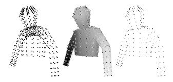
Figure 5. Removing occluded model points with the z-bufferalgorithm. Each point is compared against the z-buffer and deleted if its z-value is greater than the correspondig value in the z-buffer.
