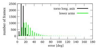
Figure 8. Distribution of tracking errors for torso longitudinal axis and lower arms.
