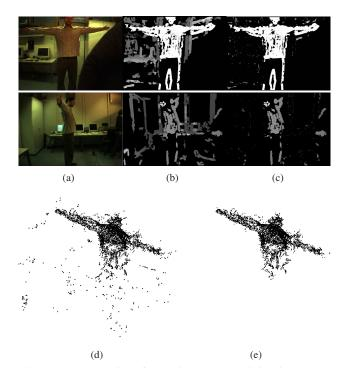
Figure 3. Preprocessing of stereo images. (a) Original images. (b) Disparity maps. (c) Result of foreground segmentation. (d) Joint point cloud in a global coordinate system. (e) Point cloud after application of noise filter.
