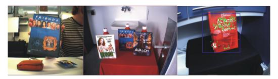
Figure 7.2: Snapshots taken from the robot camera. From left to right: object held in front of the robot's camera, multiple objects recognition, unknown object recognition during the experiment with feature extraction and shape segmentation.
