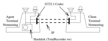
Figure 1: Typical setup for Nespole! recordings.
