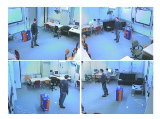
Fig. 2. Example captures of one frame from all four views in the CHIL corpus. The person recorded was to wear a magnetic motion sensor to capture his groundtruth head orientation.
