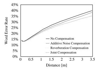
**Fig. 1.** Word error rates without compensation and with different compensation approaches for different speaker to microphone distances of a German speaker.
