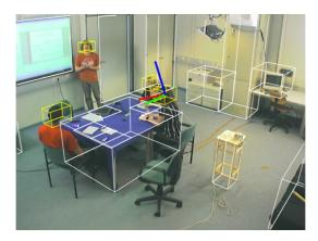
**Fig. 2.** Camera 1's view of a recorded meeting scene during a short presentation, given by person P00. Person P02, sitting opposite to the presenter, is wearing the magnetic motion sensor to capture her true head orientation, depicted by the red (x), green (y) and blue (z) coordinate axes. All *axis aligned bounding boxes* of focus targets we annotated, visible from this view, are highlighted in white.
